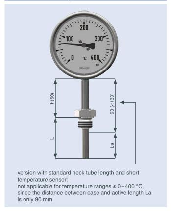
With a simple calculation it is possible to check whether the standard neck tube length h, according to the data sheet, and the requested installation length L/L1 meets the requirements regarding the minimum distance between case and La.
